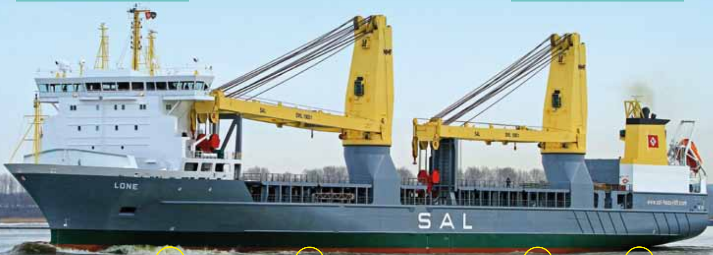
2 cranes of 1,000 mtons SWL lifting capacity each, in combination 2,000 mtons
